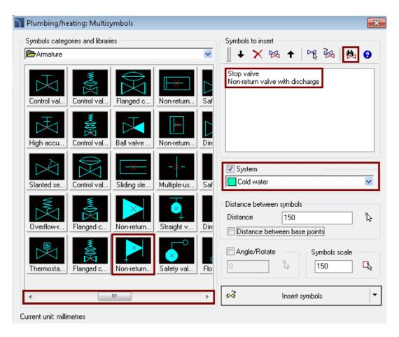
After that we click the *Insert symbols* button and we insert the chosen symbols into the line by clicking first the P1 and next the P2 point (in this way we show the direction where we would like to isnert the symbols).
