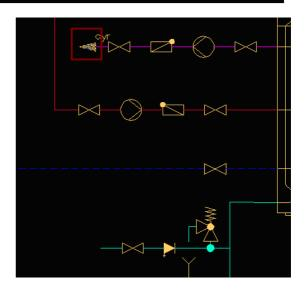
In the dialog window we need to remember to check the *Rotation* option and after that we click the *Insert symbol* button and we insert the symbol into the *Cold water* line in with right edge.
