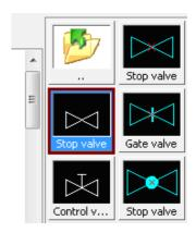
In order to choose the needed valve from the multivariant symbol we need to click into the symbol's body field and from the drop-down choose the right symbol. In our example it will be a symbol of a *Ball valve*.
