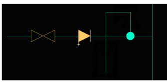
In the next step we will insert a *Overflow valve*. In order to do this we click the Cross symbols button that is located on the HVAC and Piping toolbar.
