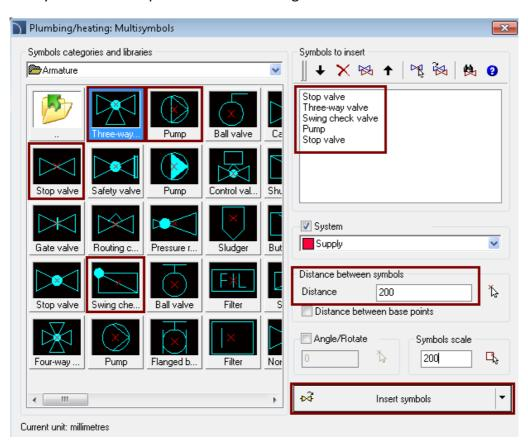
There should be a line between the symbols that's why from the *System* list we will choose *Supply* and we add the distance between the symbols as 200 in the distance box. After we have clicked the *Insert symbols* button we need to show the distributor's stub first (P1) and next we click the (P2) point in such way that the line with symbols will be drawn upwards.
