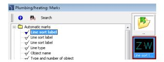
We can add marks at the same time into many lines. In order to do this we need to click the arrow that is located on the *Insert symbol* button and from the drop-down menu choose the *Into many pipes* option.
