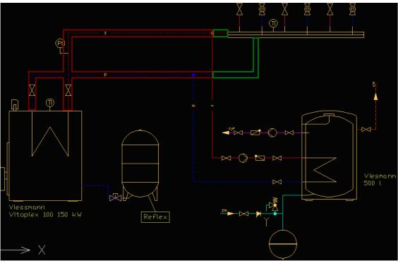
In the next step we will insert Reducers symbols. We run the *Symbols* command and using the search function search for a *Reducer*.
