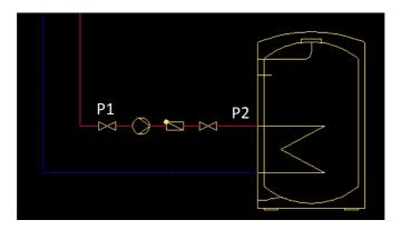
Next thanks to the *Multisymbols* command we will insert the symbols' set as we have put previously. After we have run the command we click the *Most recently selected symbols* thanks to which the last set of symbols will be added into the list (*Stop valve*, *Stop valve*, *Pump*, *Swing check valve*).
