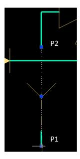
Our next task will be to insert into the drawing a *Diaphragm extension tank*. We click the *Symbols* button and we using the search function we search for the *Diaphragm extension tank*. In the parameters we check *Rotation* and we set the scale into 300 (this symbol will be bigger than the previous ones).
