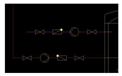
Lets insert one additional *Stop valve* on the *Return* line. We can use the *copy* option that is located in the *Quick edition* command or we can use one of the following commands:
