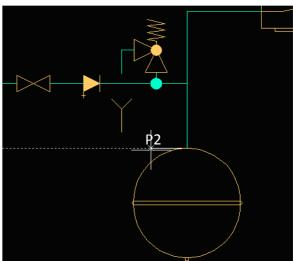
Next we will insert an *Overflow arrow* into the *Cold water* line. Because we already have this symbol inserted in our drawing we can use the *Insert similar object* command. We click the *Insert similar object* button that is located on the *CADprofi – tools* toolbar and next we select the *Overflow arrow* that was already inserted in our drawing.
