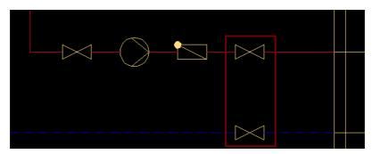
Next we will insert an *Overflow arrow* symbol on the *circulation* line. We click the *Marks* button that is located on the *HVAC and Piping* toolbar.
