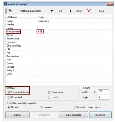
The command Attributes and descriptions 4 may be used to many symbols at the same time. After we have run the command we need to type in the command line: Multiple and after that choose the desired symbols.
