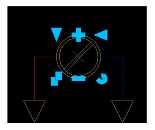
Just to give an example we will copy the *Stop valve* symbol in order to insert its copy into the *Return line*. We will run the *Quick edit* command and next we will choose the *Stop valve*. Clicking on the copying mark we will copy the symbol into a different place. Program is in the copying mode until we press the key thanks to this we can insert many copies of our selected symbol.
