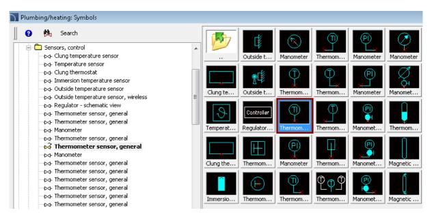
We set the scale as 200 and we insert the *thermometer* symbol into the boiler.
