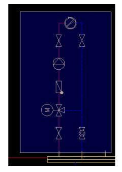
After we have ended choosing the objects that we would like copy we select the base point to copy (P1) and next we click on the P2 point (or next points) in which we would like to put the copy of the selected objects.
