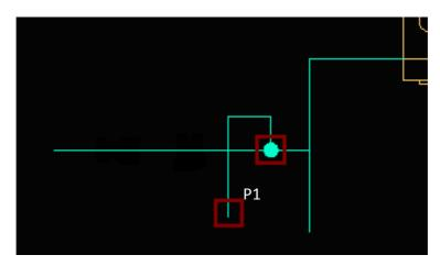
Our next step will be to insert two symbols into the water line. We run *Multisymbols* command. From the *Armature* category we choose the *Stop valve* and the *Non-return valve* with discharge (we can find it using the search button). Additionally we set the distance and the scale to 150.
