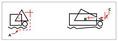
To stretch entities, select them using a crossing window (A) or crossing polygon, and then specify the base point (B) and displacement point (C).
