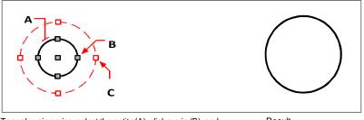
To scale using grips, select the entity (A), click a grip (B), and scale the entity by dragging the grip to its new location (C).
