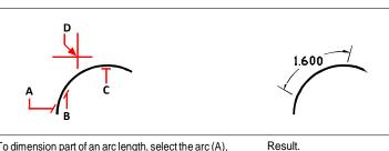
To dimension part of an arc length, select the arc (A), select the start point (B) and end point (C) of the portion to measure, then specify the dimension arc location (D).
