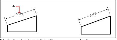
Select the dimension to be rotated (A), and then type the rotation angle.
