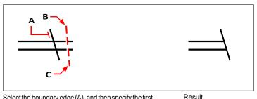
Select the boundary edge (A), and then specify the first point (B) and second point (C) of the fence.
