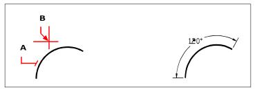
To dimension the angle subtended by an arc, select the arc (A), and then specify the dimension arc location (B).
